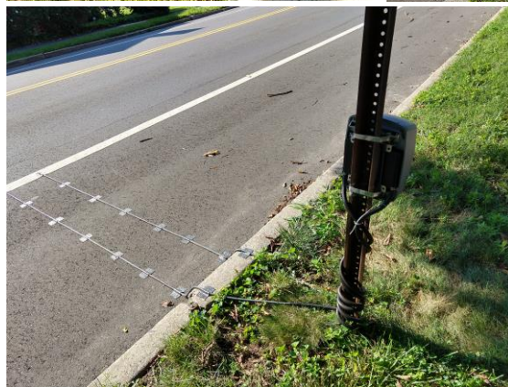
Counter locations on the east (top left) and west (top right) sides of Main Street, and the counter and tubes installed (bottom).
